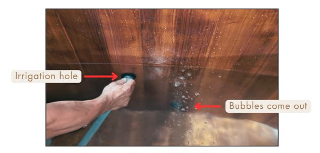
After 1-2 minutes of water injection, and no air bubbles are coming out of the water outlet, the hose can then be removed, as shown below.
